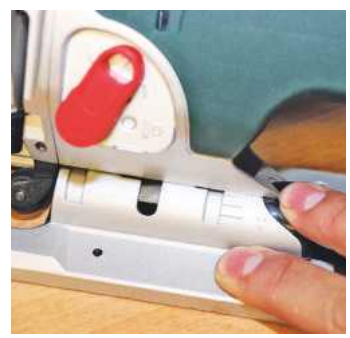
▲ The edge of the base aligns to the etched markings for setting to common angles
